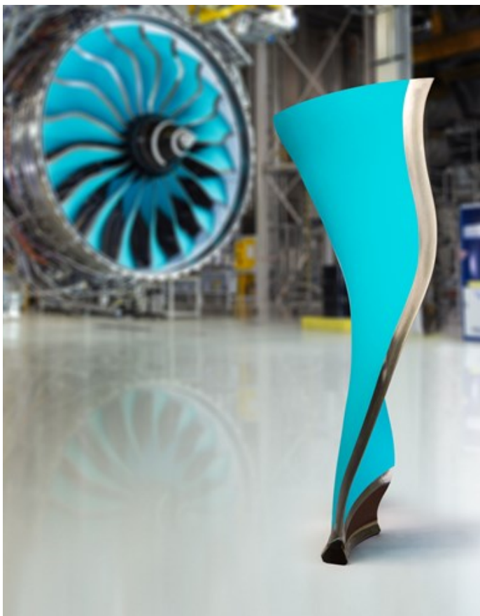
FIGURE 5: Photo of the UltraFan Turbine Blade, Showcasing the Titanium Leading Edge With the Full UltraFan Engine in the Background [49].
